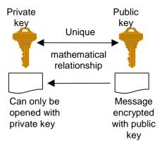
A transaction submitted by a customer to an online merchant via the Internet can be encrypted with the merchant's public key and therefore can only be decrypted by that merchant using the merchant's private key—ensuring a level of confidentiality. Confidentiality can also be achieved through the use of Secure Socket Layer (SSL), Secure/Multipurpose Internet Mail Extensions (S/MIME), and other protocols, such as Secure Electronic Transaction (SET).
